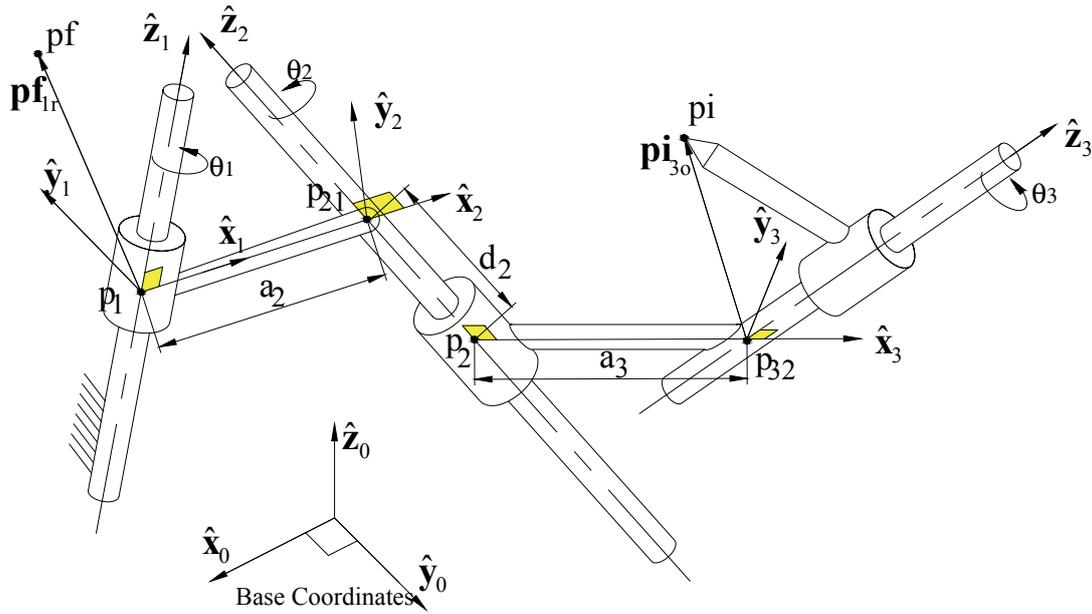
Figure 2. A General View of a 3R Manipulator Arm at Its Zero Position.
