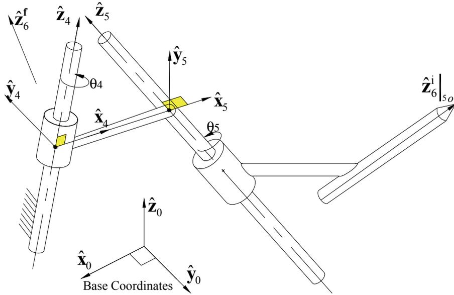
Figure 4. A 2R Arrangement Used for Orienting Vectors in Space.
