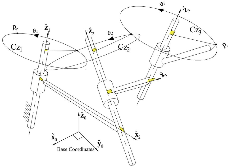
Figure 3. The Kinematic Behaviour of the Arm Joints.
