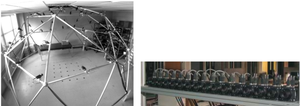
Figure 6. Example of convergent setup with 51 cameras proposed in [26] (left) and a parallel one with 16 cameras in [43] (right).
