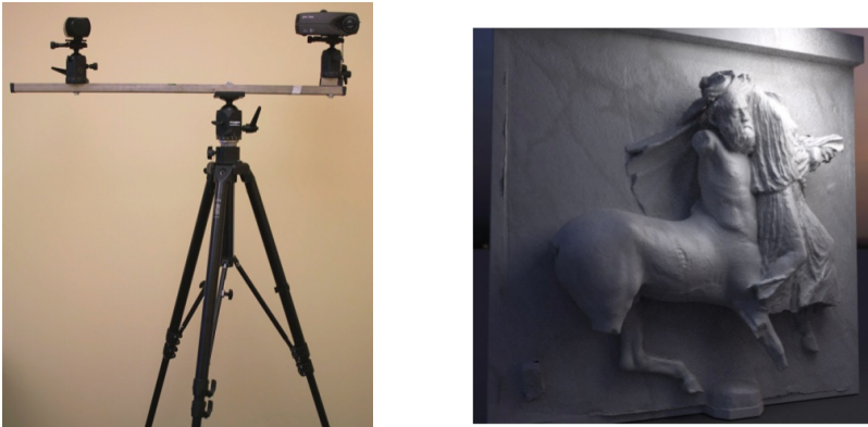
Figure 5. Simple structured light scanner consisting of a digital camera, a projector and a tripod used in [73] and, on the right, a sculpture model obtained after 14 scans.
