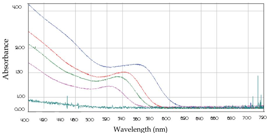
Fig. 4. UV-Vis spectra of Cd-Se colloidal suspension
