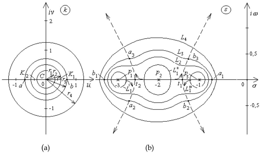
Figure 6. Circular root locus field when setting the image center in the origin of the variable parameter plane  $k$
