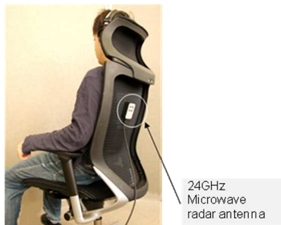
Fig. 1. Prototype chair equipped with a non-contact microwave radar system to monitor mental stress in workers (Suzuki et al., 2008).
