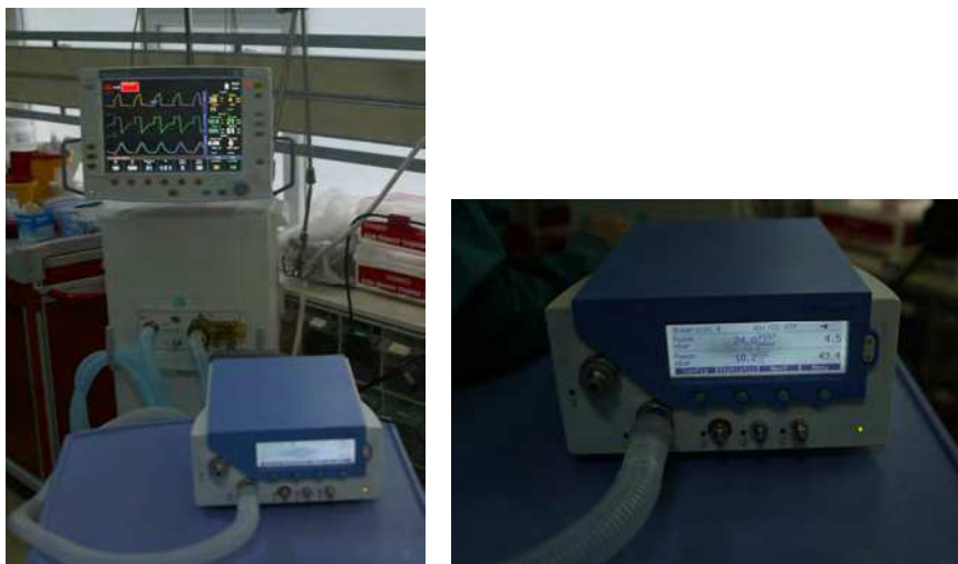
Fig. 12. The performance measurement of the anesthesia machine
