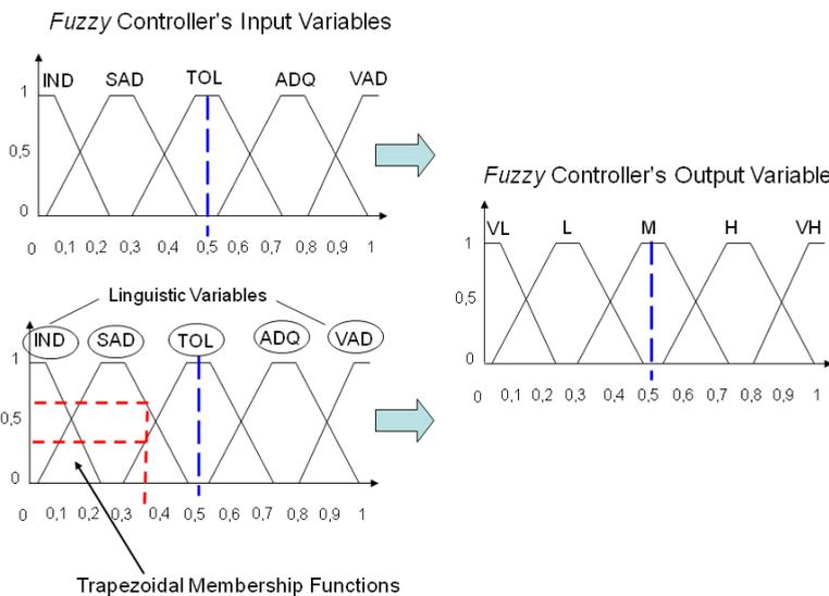
Fig. 2. Input controller's input and output membership functions
