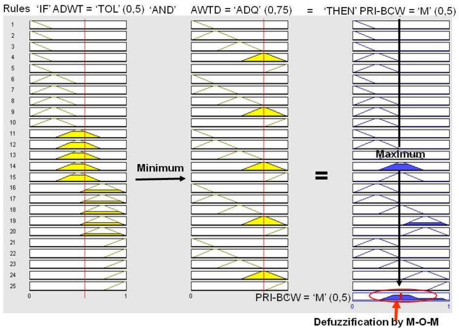
Fig. 3. The steps of fuzzy inference and defuzzification for the input controller
