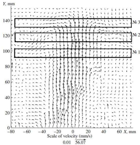
Fig. 8. Velocity field of buoyant turbulent jet.
