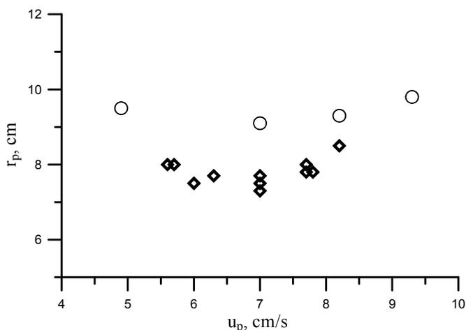
Fig. 13. Experimental jet parameters (maximum longitudinal velocity and radius): ○ – calculated in the framework of the integral model for discharge rates of buoyant jets 40, 70, 100 and 150 cm/s; ◇ – parameters, measured in the experiments with one jet.
