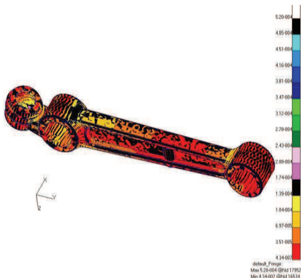
Fig. 5. Stress distribution and strain gauge positions
