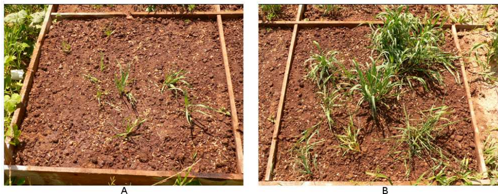
Fig. 11. Pilot testing: soil phytotoxicity evaluation. June, 2007. A – Control plot (soil with oil), B – Plot 4 pre-treated with the consortium "MicroBak" and a fertilizer
