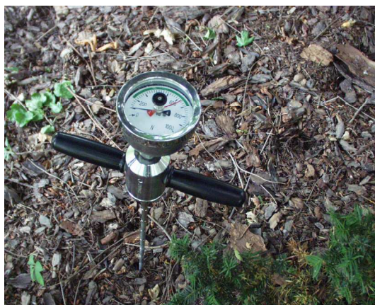
Fig. 7. Measurement of soil resistance by penetrometer
