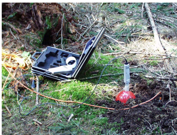
Fig. 4. Upper panel - Concentration of CO 2 in soil air in a crossing line after several harvester passages (soil moisture: 35%). Lower panel - CO 2 measurement in control line with GMP 221 Carbon dioxide probe (Vaisala, Finland)
