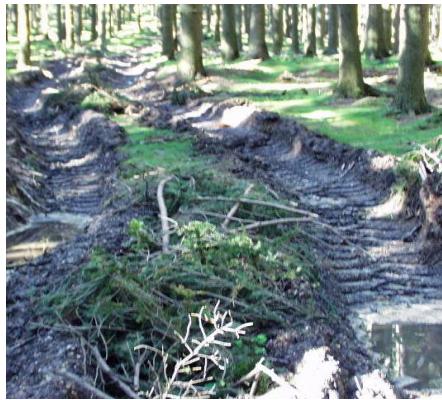
Fig. 6. A case of rut depth up to 25 cm, which is a point when an ecological risk may appear.
