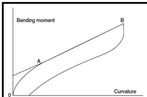
Fig. 3. Typical bending curve of woven fabrics (Schwartz, 2008)
