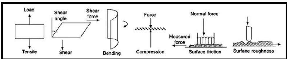
Fig. 7. Measuring principles of the KES system
