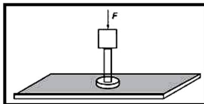
Fig. 10. Compression test on the KES-F system (Hu, 2008)
