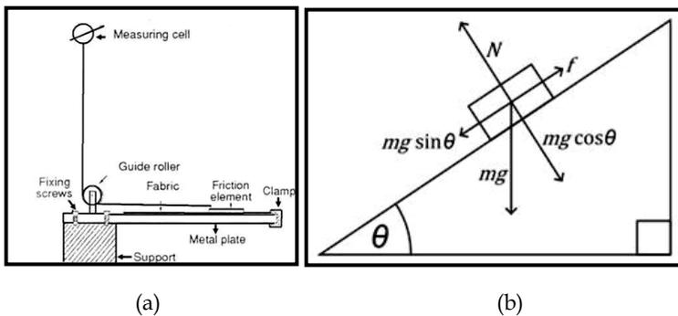
Fig. 17. Basic fabric friction measurement methods (Bona, 1994)
