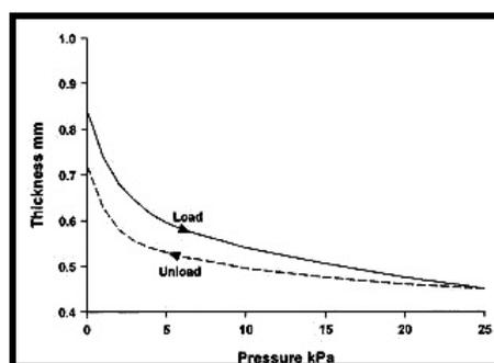
Fig. 5. The change in thickness with pressure (Saville, 1999)
