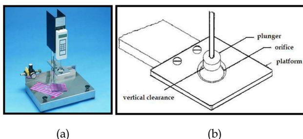
Fig. 15. (a) Circular bending rigidity tester ([www.sdlatlas.com](http://www.sdlatlas.com)), (b) Platform and plunger of the tester (ASTM D 4032 - 08)
