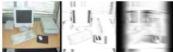
Figure 2. Example image (left). Vertical symmetry image calculated with small operator ( m = 10 ; centre) and with large operator ( m = 50 ; right). Brightness corresponds to symmetry.
