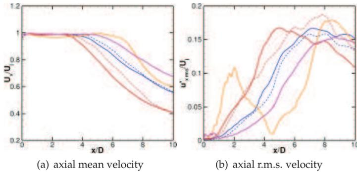
Fig. 12. Simulated axial (a) mean and (b) r.m.s. velocity on jet axis. Isothermal jets: – baseline; – – continuous microjets; –  $f_F = 3$  kHz pulsed microjets; –  $f_F = 9$  kHz pulsed microjets. Heated jets: - - baseline; - - - continuous microjets.
