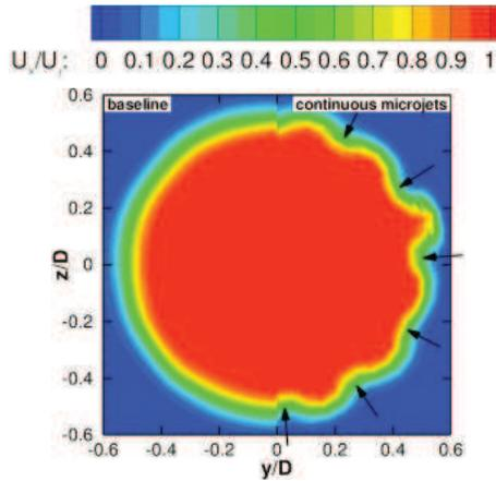
Fig. 7. Mean axial velocity computed at  $x/D = 1$  for the baseline (left) and continuous microjets (right) isothermal configurations. Arrows represent the position of the microjets.
