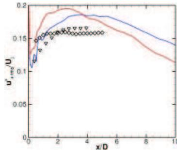
Fig. 5. Evolution of the axial r.m.s. velocity  $u'_{rms}$  along the nozzle lip. Simulations: – isothermal and – heated baseline configurations. Measurements:  $\diamond$  Husain and Hussain for an initially turbulent shear layer (Husain & Hussain, 1979) and  $\nabla$  Fleury et al. for a Mach 0.9 jet at  $Re_D = 7.7 \times 10^5$  (Fleury et al., 2008).
