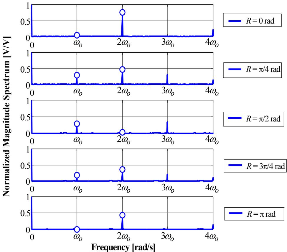
Fig. 7. Normalized frequency spectra of the interferometer signal described by Eqn. (7) at five different values of the phase  $R$ . The open circles represent the values of the fundamental and second harmonic frequency components.
