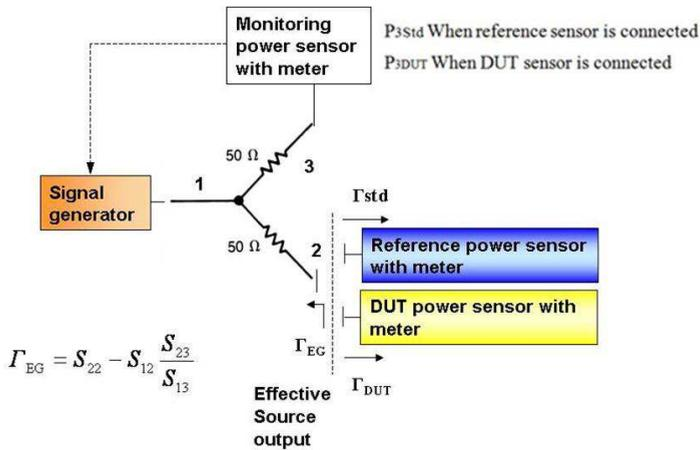
Fig. 4. Coaxial splitter based power measurement setup
