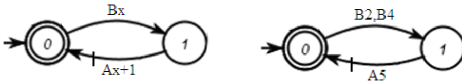
Fig. 8. "E" specifications for B_A , B_B and B_D , buffers (on the left) and B_C (on the right)
