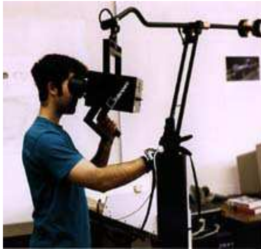
Fig. 2. A binocular omni-orientation monitor (BOOM)
