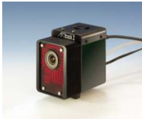
Fig. 4. A.R.T. optical tracking system
