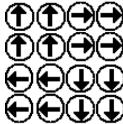
Fig. 14. Ordering of the atomic dipoles in a superparamagnetic material.
