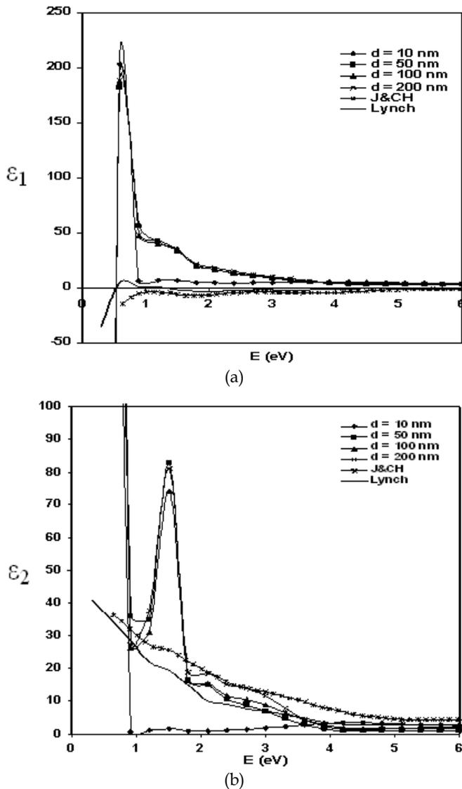
Fig. 1. The dielectric constants of deposited TiO<sub>2</sub>/glass films of Different thicknesses at 473 k (a) Real part (b) Imaginary Port.
