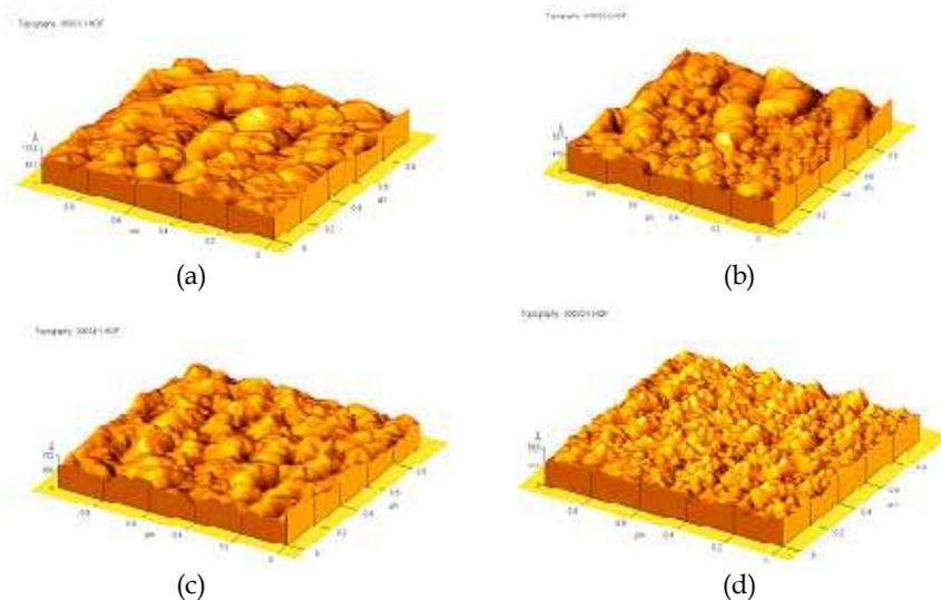
Fig. 8. The topography of TiO<sub>2</sub> / glass with (a)20 nm, (b)70 nm, (c)200 nm, (d)250 nm thickness at 600 k.
