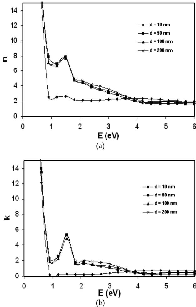
Fig. 4. Refractive index Vs. energy for different film thicknesses deposited  $\text{TiO}_2/\text{glass}$  films at 473 K, (a) Real part (b) Imaginary part.
