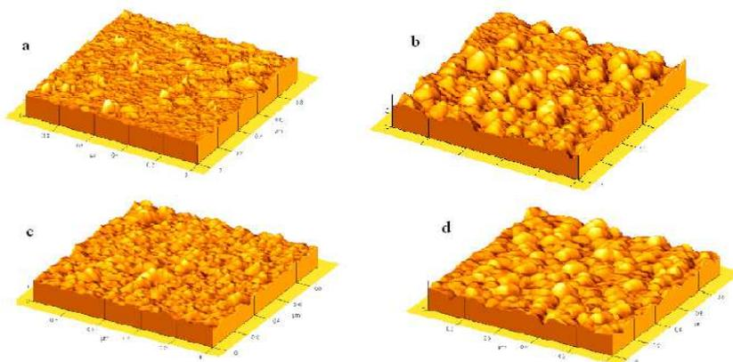
Fig. 5. The topography of  $\text{TiO}_2$  / glass with (a)10 nm, (b)50 nm, (c)100 nm, (d)200 nm thickness at 473 k.
