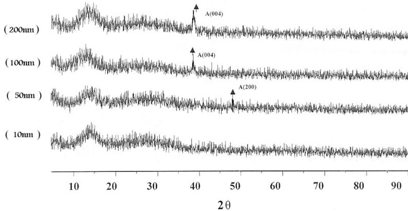
Fig. 7. The XRD pattern of TiO<sub>2</sub> / glass layers with different thicknesses at 473 k.
