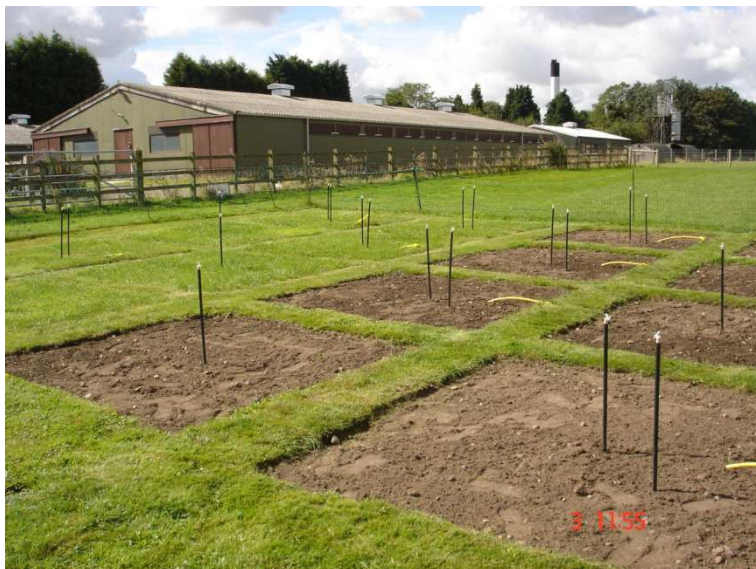
Photo 1. The ASgard site. Both pasture and fallow plots with gassing pipes and measuring tubes can be seen.
