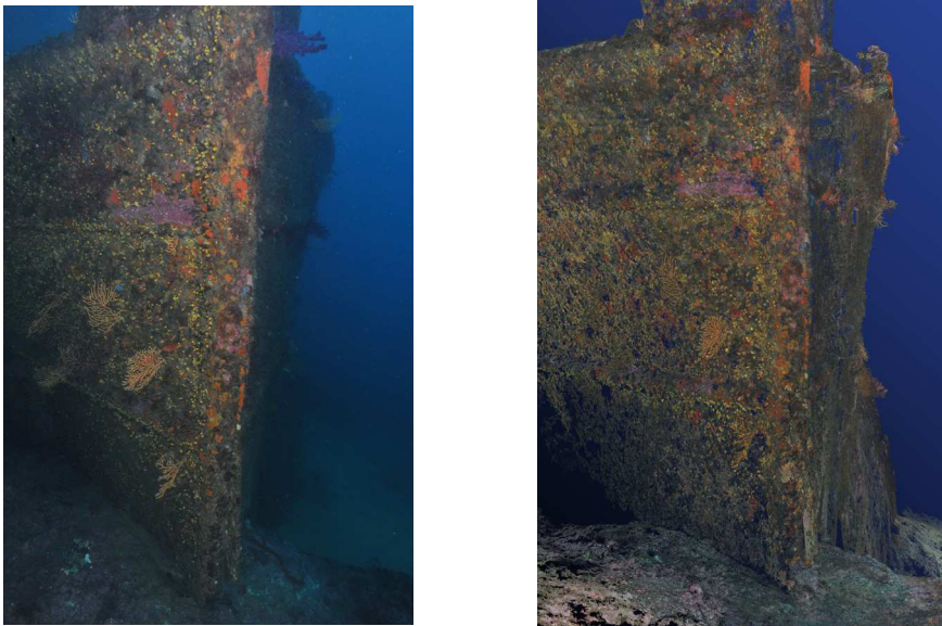
Fig. 17. On the left, one of the 1,828 digital photographs taken. On the right, the Liban wreck: cloud of 3D points measured by photogrammetry using the Furukawa method.
