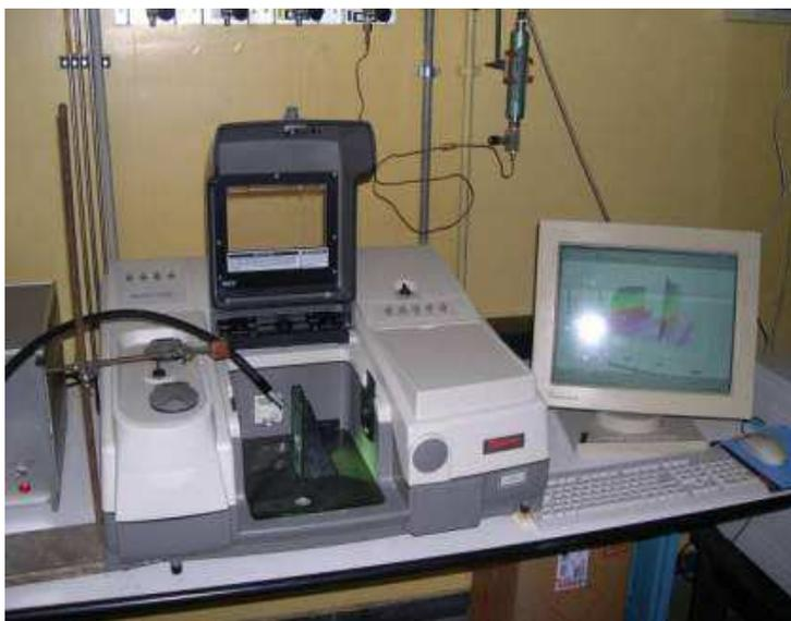
Fig. 1. Set up for RT-FTIR monitoring of UV irradiation curing
