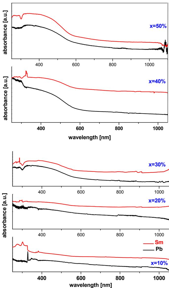
Fig. 3. UV-VIS absorption spectra of  $x\text{PbO}$  (or  $x\text{Sm}_2\text{O}_3$ )· $(100-x)[3\text{TeO}_2\cdot 2\text{V}_2\text{O}_5]$  samples where  $0 \leq x \leq 50\text{mol}\%$  in function of lead (II) or samarium (III) oxide content.
