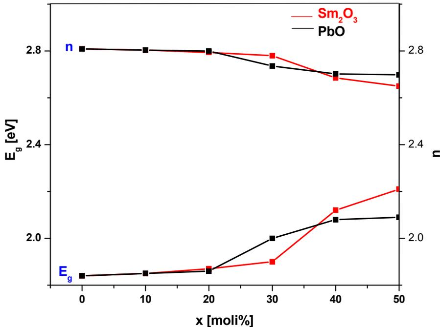
Fig. 6. The relationship between the optic gap,  $E_g$ , and refractive index,  $n$ , and the and the PbO or Sm<sub>2</sub>O<sub>3</sub> contents (the line is only a guide for the eye).
