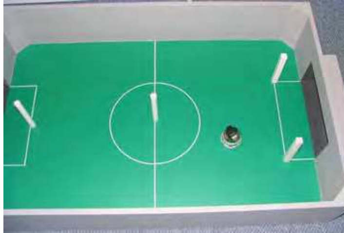
Figure 15. Experimental setup, the landmarks are the vertical tubes
