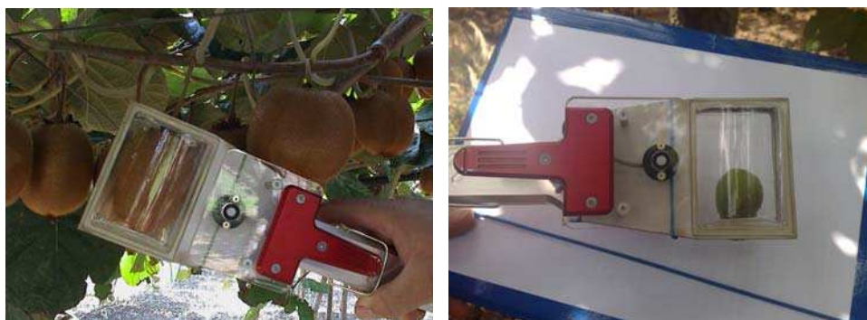
Photo 1. Measurement of fruit transpiration in attached kiwifruit (left) and detached apricot (right) using a portable gas-exchange equipment (ADC-LCA4, ADC BioScientific Ltd, Hoddesdon, England).
