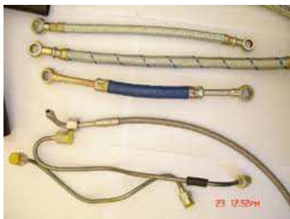
Fig. 25. Alodine coated Fuel Injection Fuel Lines
