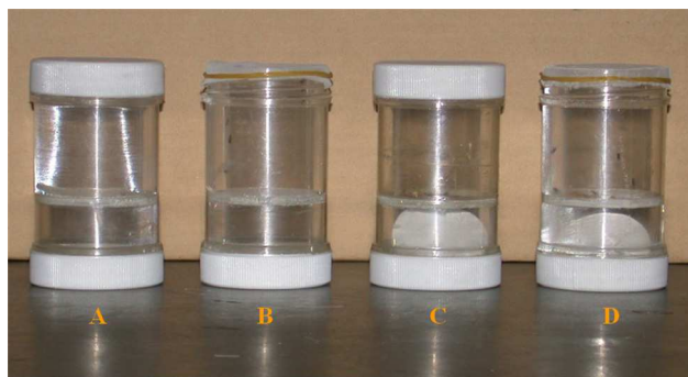
Fig. 3. Bioassay system used for fumigant test of allyl and butyl isothiocyanates against four stored products insect pests.
