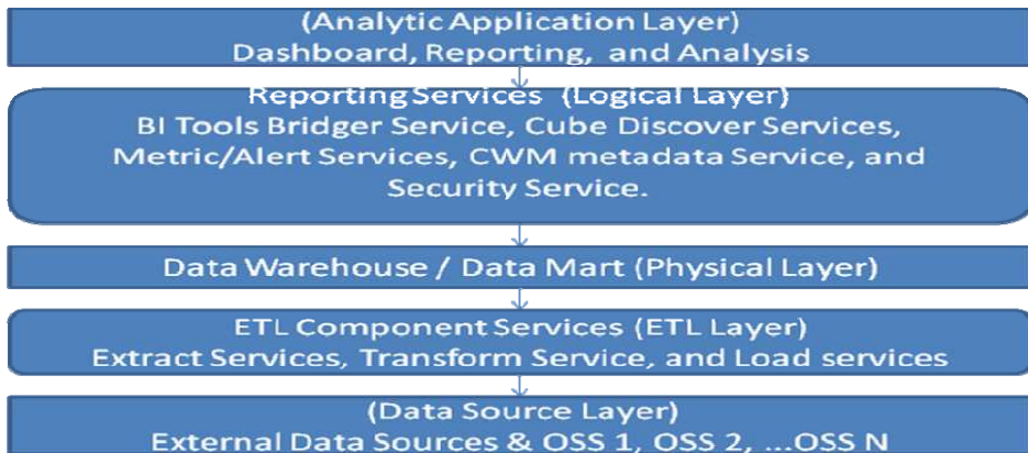
Fig. 4. Current BI Architecture (Wu et al, 2007)
