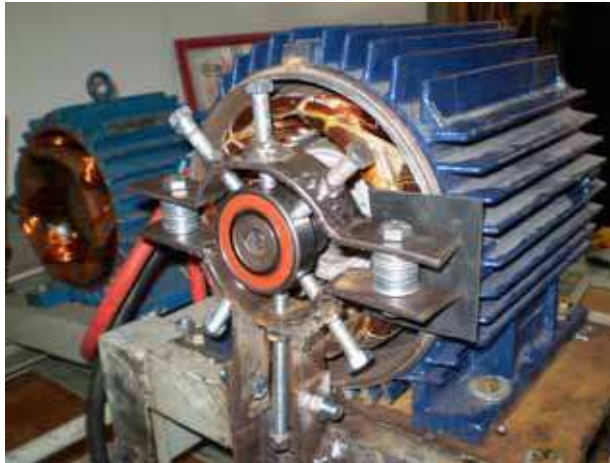
Fig. 14. Eccentricity induced failure
