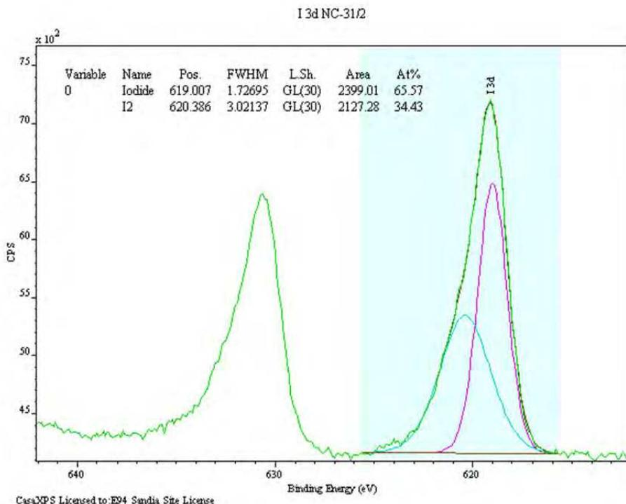
Fig. 8. X-ray photoelectron spectra (XPS) showing 66% of  $I_2$  converted to I<sup>-</sup> upon iodine sorption onto Ag-alumina nanoporous material.
