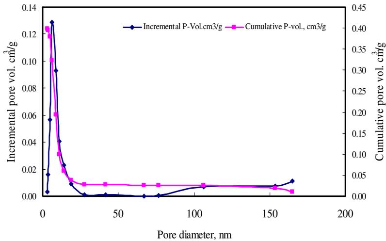
Fig. 3. Pore size distribution of Ni-Al (Ni:Al = 1:1) nanoporous material determined from BET measurements.
