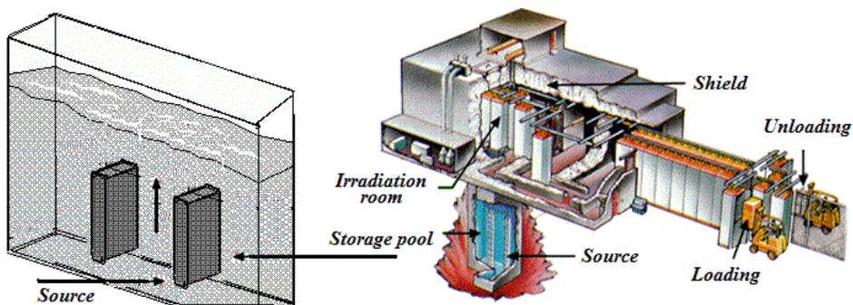
Fig. 1. Schematic diagram of a commercial gamma irradiator. The sealed sources are stored in water and raised into the air to irradiate a product that may be moved into the irradiation room on a conveyor system.
