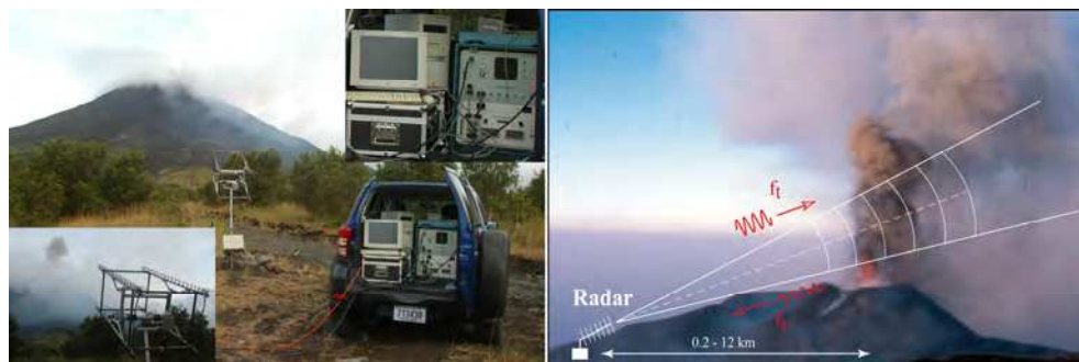
Fig. 4. (left): The transportable volcano Doppler radar VOLDORAD 2 deployed at Arenal. The PC and radar in the car trunk are connected to the antenna system via a switch box and fed by a small generator. Upper inset : Radar with PC for data storage and real-time monitoring and GPS receiver for time synchronization; lower inset : antenna (square array of Yagi) aiming at the summit to sound ash emissions. Photos: courtesy of S. Valade, OPGC (2009).
