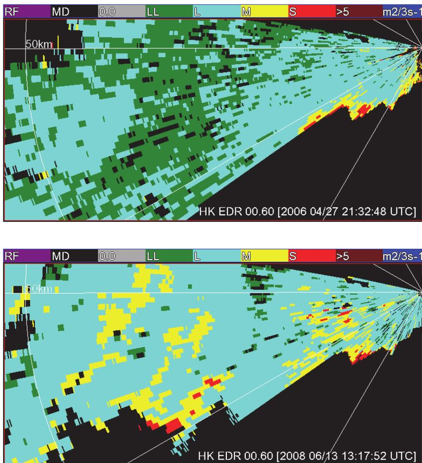
Fig. 10. EDR maps (a) at 21:32 UTC on 27 April 2006 and (b) 13:17 UTC on 13 June 2008. The mountainous Lantau Island is located to the south of the radar scans.
