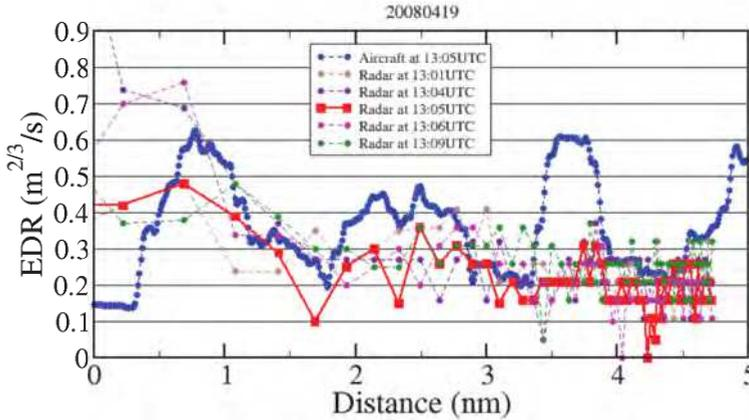
Fig. 13. EDR along the flight path estimated by the aircraft B777 (blue dots) at 13:05 UTC and by the TDWR radar at the time indicated in the legend on 19 April 2008. X axis is the distance between aircraft and the end of runway. The distance interval shaded by the green color indicates where the aircraft passes through the altitude interval observed with the  $0.6^\circ$  elevated beam.
