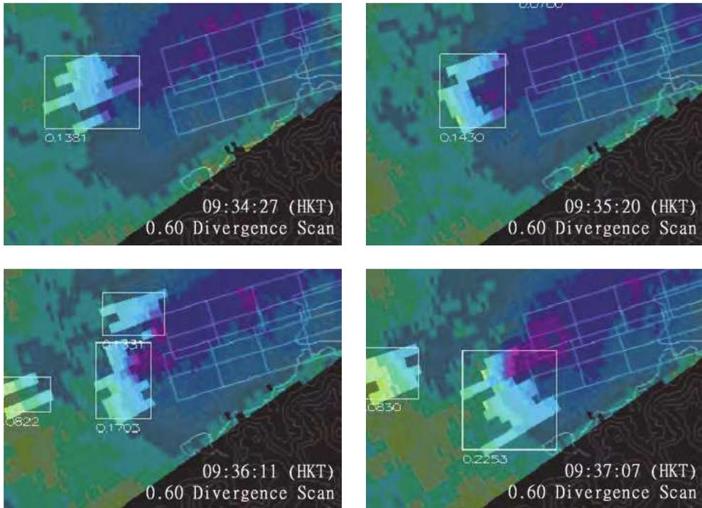
Fig. 7. Time series of the divergence feature associated with a microburst on 8 June 2007. The feature is highlighted in lighter colour and enclosed in a box. The number next to the box is the F-factor calculated for the feature. The background is the radial velocity from the TDWR, with the colour scale given in Figure 6.
