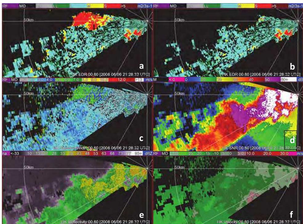
Fig. 9. (a) EDR, (b) EDR with SNR > 20 dB, (c) spectrum width, (d) SNR, (e) reflectivity, and (f) Doppler velocity at elevation angle of  $0.6^\circ$  at 21:28 UTC on 6 June 2008. Range ring is 50 km and azimuths are every  $30^\circ$ .
