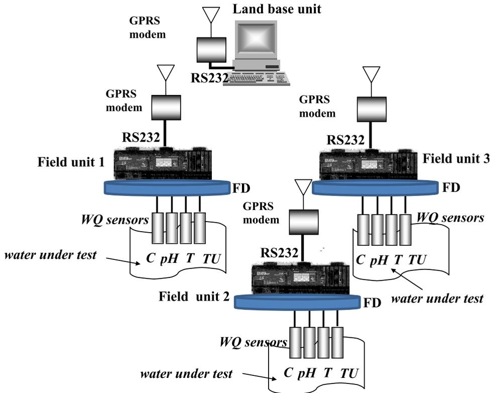
Fig. 8. Water quality (WQ) monitoring architecture based on FieldPoint embedded systems and GPRS modems.
