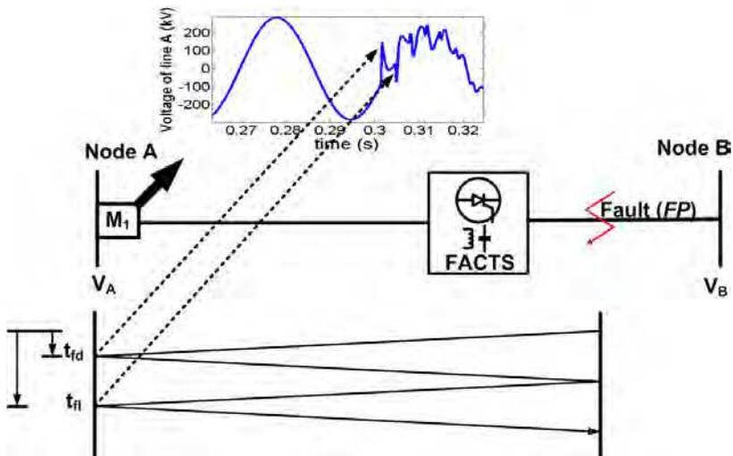
Fig. 25. Path of traveling wave due to fault
