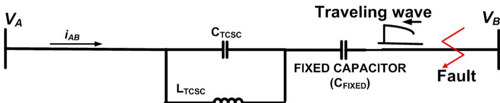
Fig. 16. Traveling wave when Thyristor is closed
