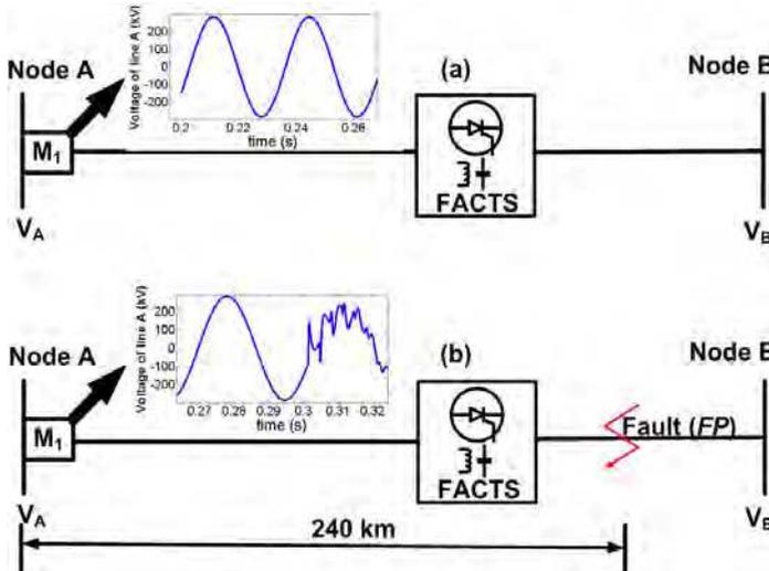
Fig. 24. Signals monitored by  $M_{1r}$  before and after a fault
