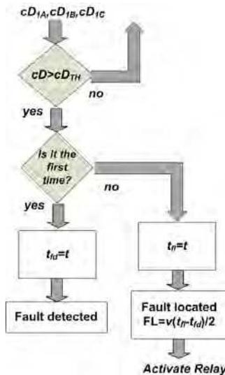
Fig. 23. Procedure to detect and locate fault
