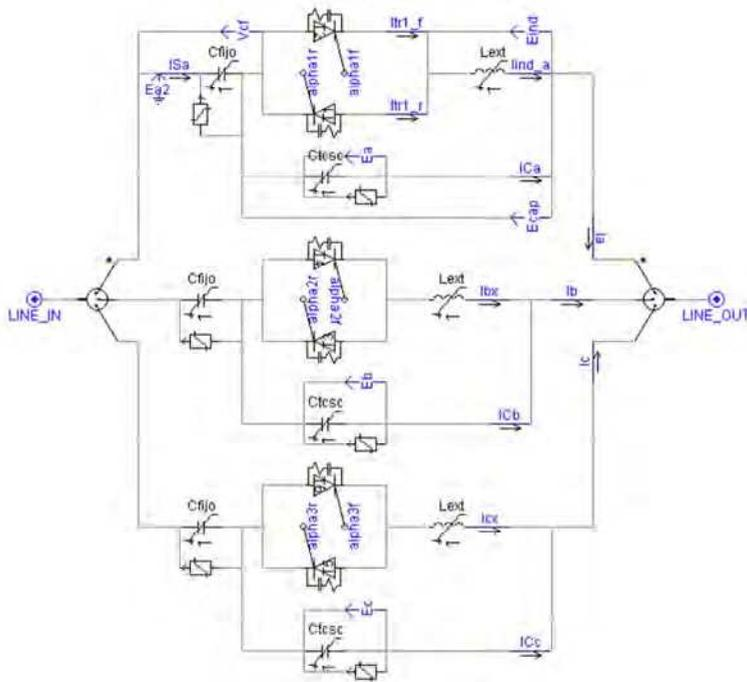
Fig. 28. TCSC configuration for the case study
