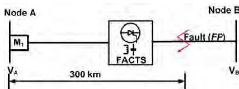
Fig. 18. Three phase to ground fault at 300 km.
