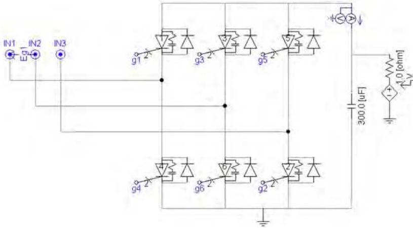
Fig. 27. SSSC configuration for the case study
