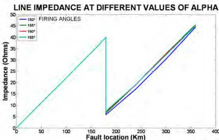
Fig. 10. Line impedance with TCSC after a fault.
