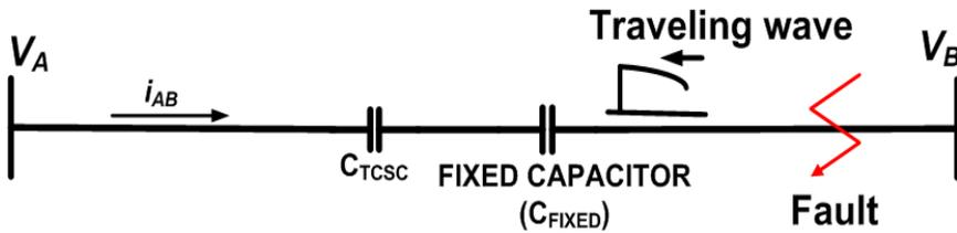
Fig. 15. Traveling wave when Thyristor is open
