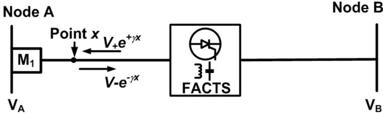
Fig. 13. Voltage in any point along the line
