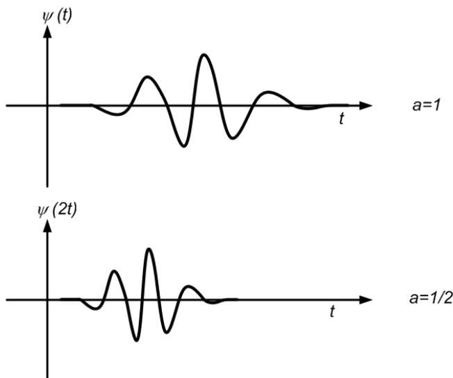
Fig. 1. Scaling the wavelet signal
