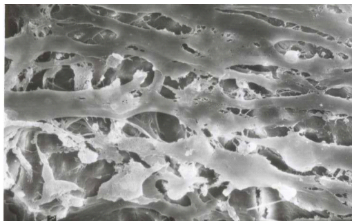
Fig. 5. The co-cultured cell compound with the material (scanning electron microscope, 1000x)
