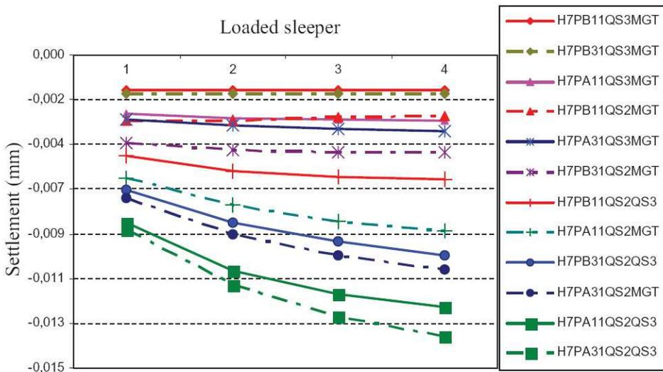
Fig. 11. Deflection of the head of loaded rails
