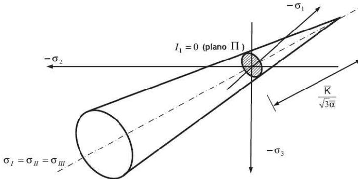
Fig. 8. Schematic of yield surfaces Drucker-Prager
