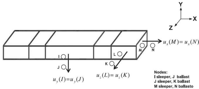
Fig. 6. Schematic of the ballast-sleeper contact
