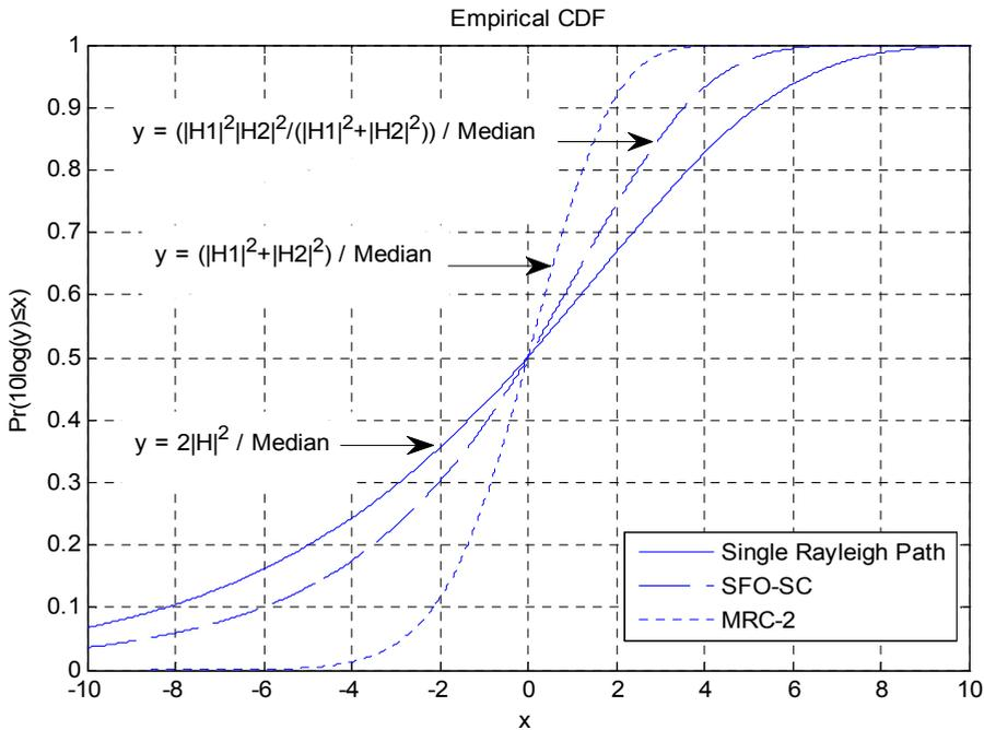
Fig. 2. Diversity gain from Symmetric Combination
