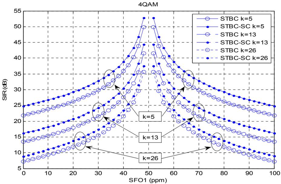
Fig. 9. SIR for Different SFO1/SFO2 ( $k=5/13/26$ ,  $m=50$ )
