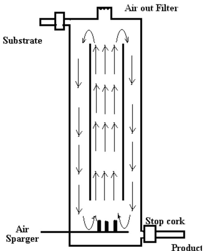
Fig. 4. Internal air-loop reactor for Cephalosporin C production
