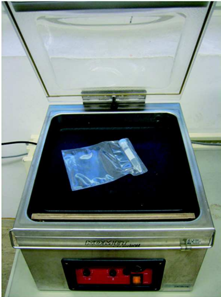
Fig. 2. Vacuum sealing device (Komet, Plochingen, Germany).
