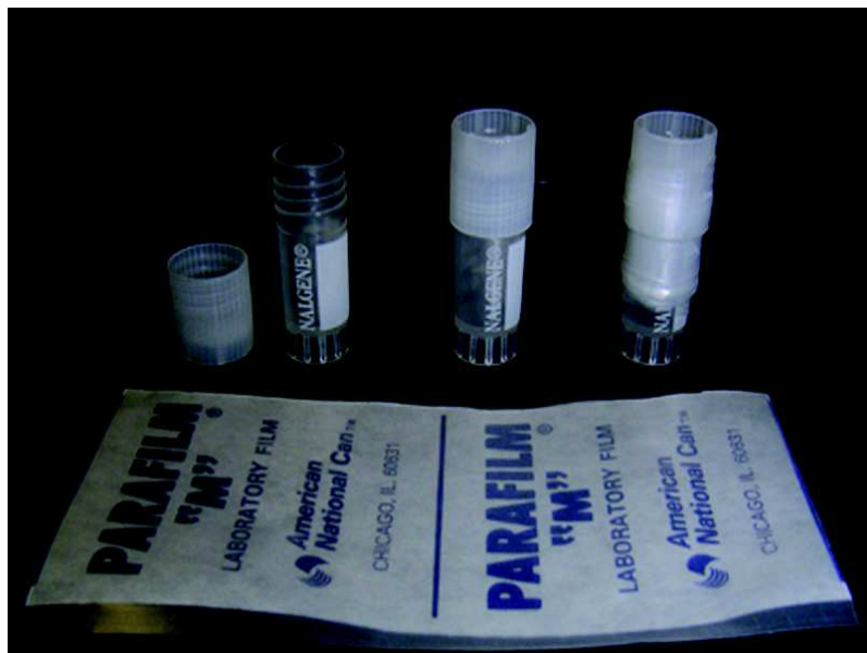
Fig. 3b. 2 ml Nalgene cryogenic vials (Thermo Fisher Scientific, Wiesbaden, Germany) (3b), filled with Ringer buffer and tightly sealed (e. g. with parafilm, American National Can GmbH, Gelsenkirchen, Germany).
