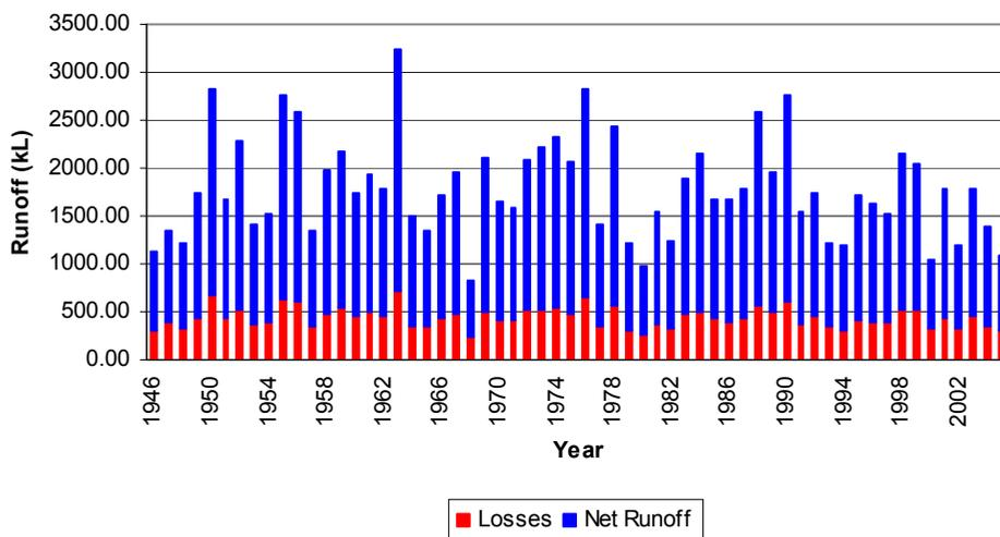
Fig. 8. Loss and runoff (4,000m<sup>2</sup> site area)
