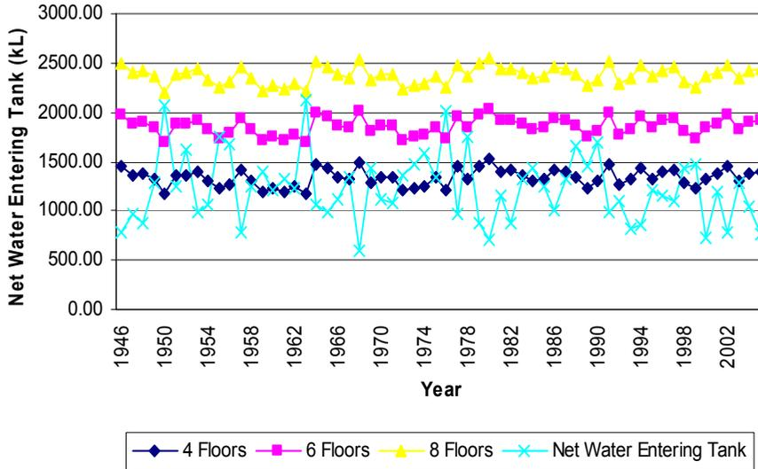
Fig. 13. Water entering tank vs. water demand (Non-BASIX and 4,000m<sup>2</sup> site area)
