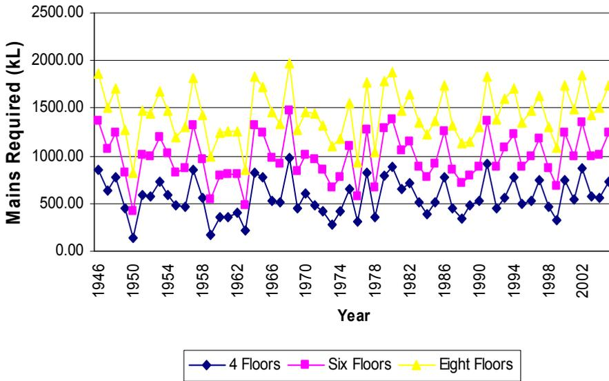
Fig. 17. Mains top-up required vs. water demand (Non-BASIX and 4,000m<sup>2</sup> site area)
