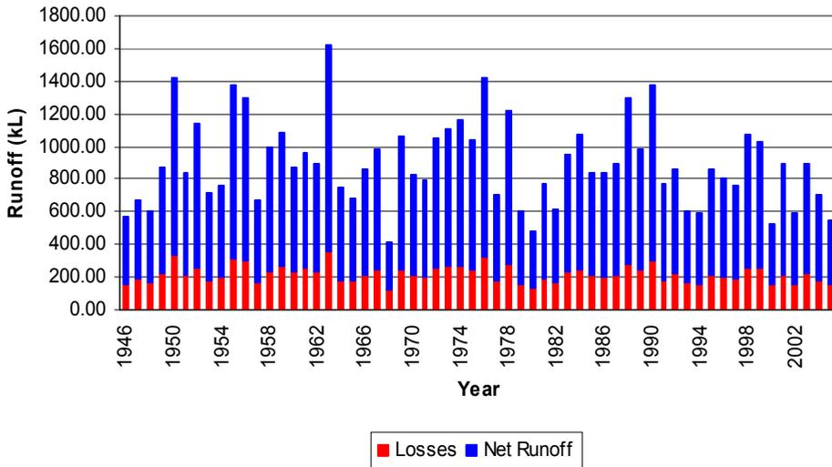
Fig. 7. Loss and runoff (2,000m<sup>2</sup> site area)
