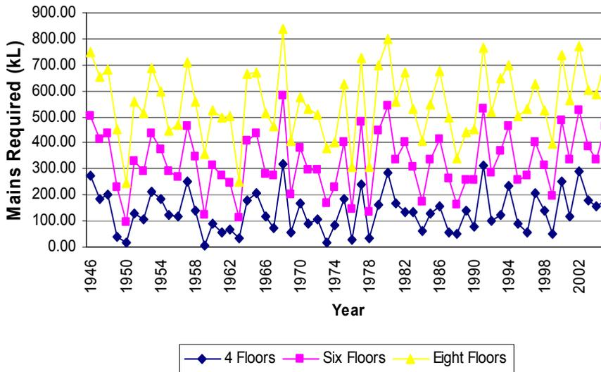
Fig. 14. Mains top-up required vs. water demand (BASIX and 2,000m<sup>2</sup> site area)
