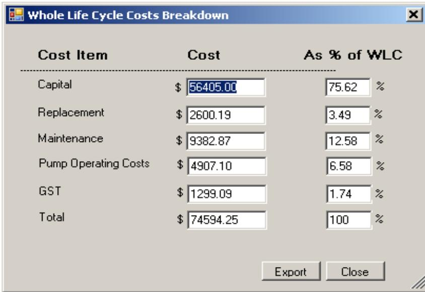
Fig. 4. Whole life cycle (WLC) cost breakdown as an output from the RWTAM program
