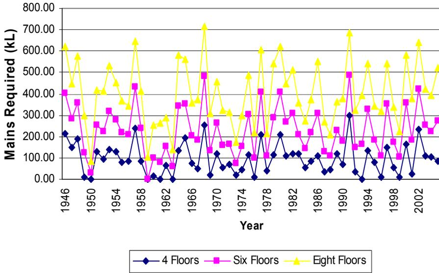
Fig. 15. Mains top-up required vs. water demand (BASIX and 4,000m<sup>2</sup> site area)
