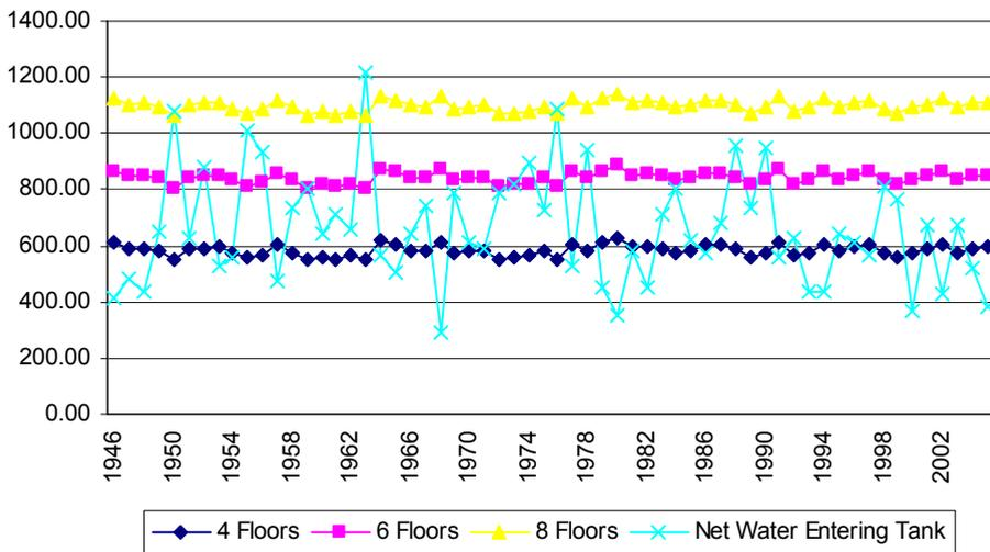
Fig. 10. Water entering tank vs. water demand (BASIX and 2,000m<sup>2</sup> site area)
