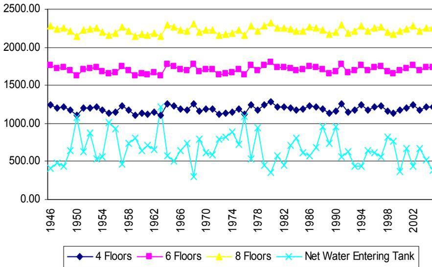
Fig. 11. Water entering tank vs. water demand (Non-BASIX and 2,000m<sup>2</sup> site area)
