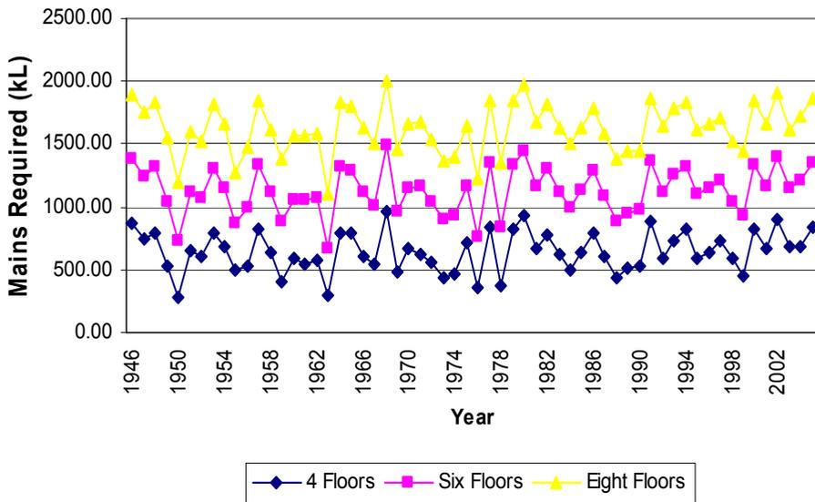
Fig. 16. Mains top-up required vs. water demand (Non-BASIX and 2,000m<sup>2</sup> site area)
