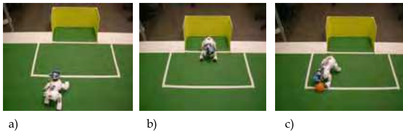
Figure 11. Basic goalie behaviors: a) Goalie-return-to goal, b) Goalie-position, c) Goalie-clear ball. For each behavior a different vision system is used and a different particle filter setting
