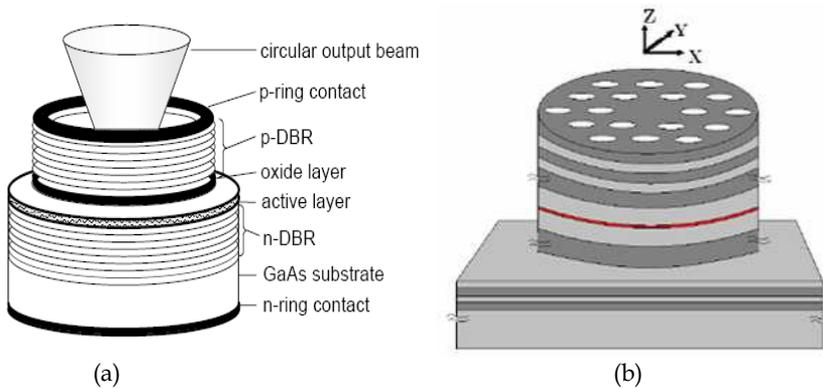
Fig. 1. VCSEL structure ((a): conventional VCSEL, (b): PhC-VCSEL)
