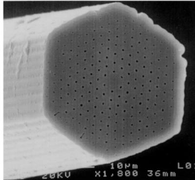
Fig. 4. Photonic crystal fiber
