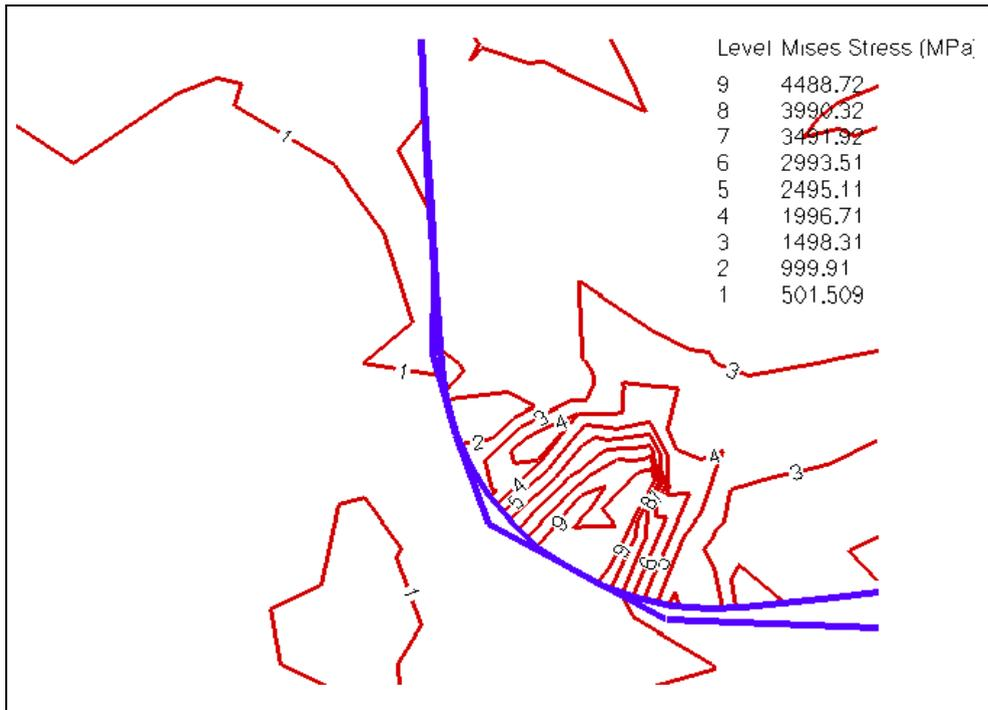
Fig. 3. Von mises stress for simulation no.9.
