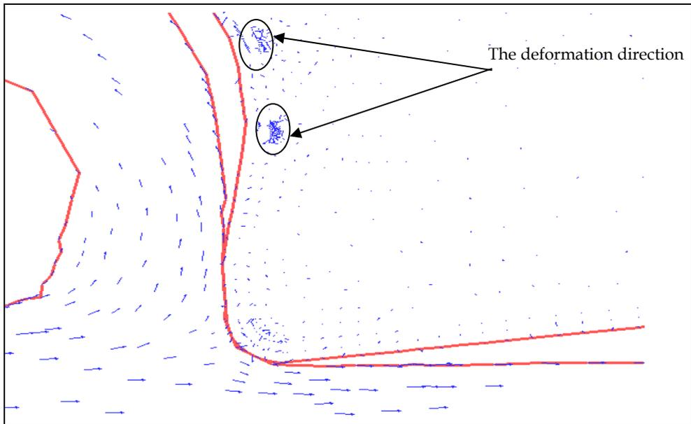
Fig. 5. The velocity vectors for simulation no.9.
