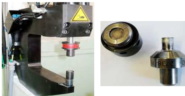
Fig. 11. Clinching machine and clinching tools.
