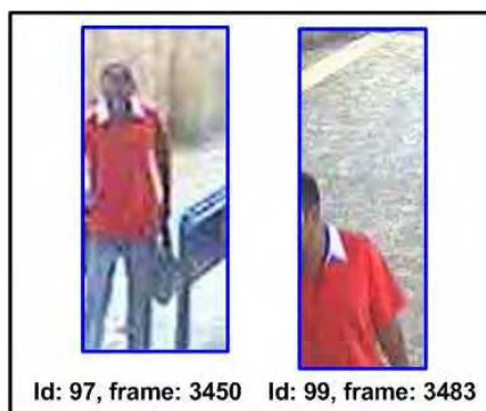
Fig. 7. An example of the object ID persistence problem: two tracked objects created for one sole ground-truth object (object ID persistence = 2).
