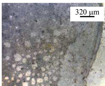
Fig. 9. Micrograph of ZA27 - 8%SiC sample after EIS test.
