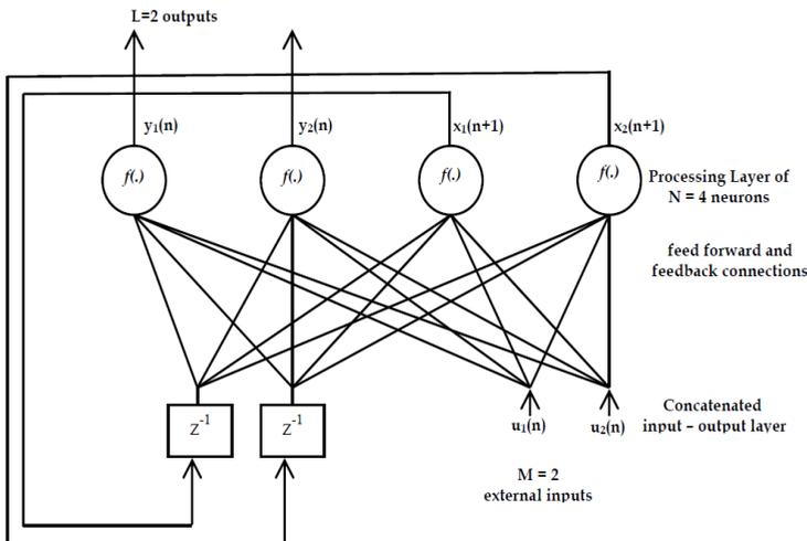
Fig. 4. Example of a partially recurrent neural network
