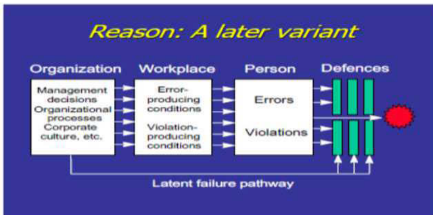
Fig. 2. A reference Model for Accident Analysis. Sourced from (Wikipedia 2011).
